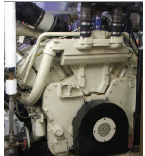
The heart of the rebuild, K38-M Tier 2 main engines.
